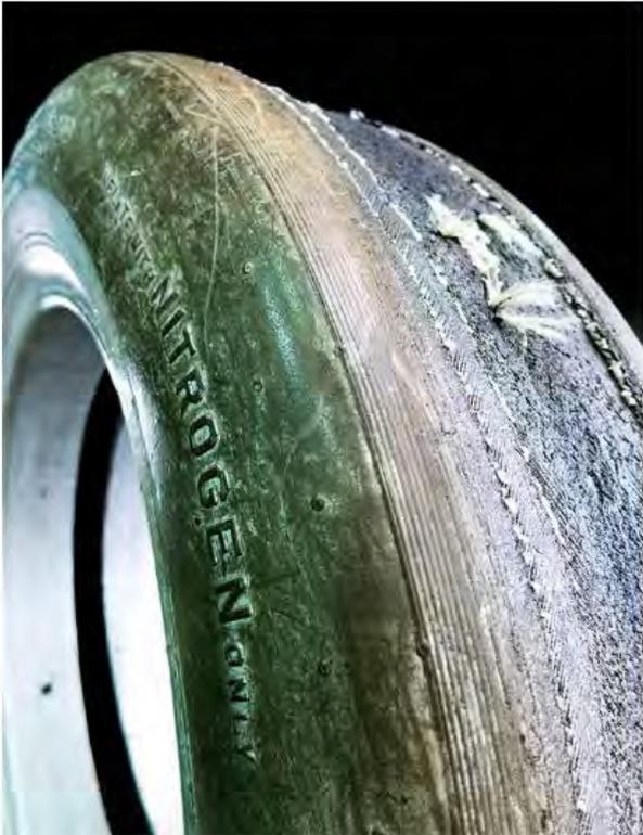
*Tires were compounded with aluminum powder to reflect heat, and filled with inert nitrogen to prevent their combustion. Made by B.F. Goodrich, tires lasted fewer than 20 landings, and cost about \$2,300 each. (Curt Mason/Project Habu)*
