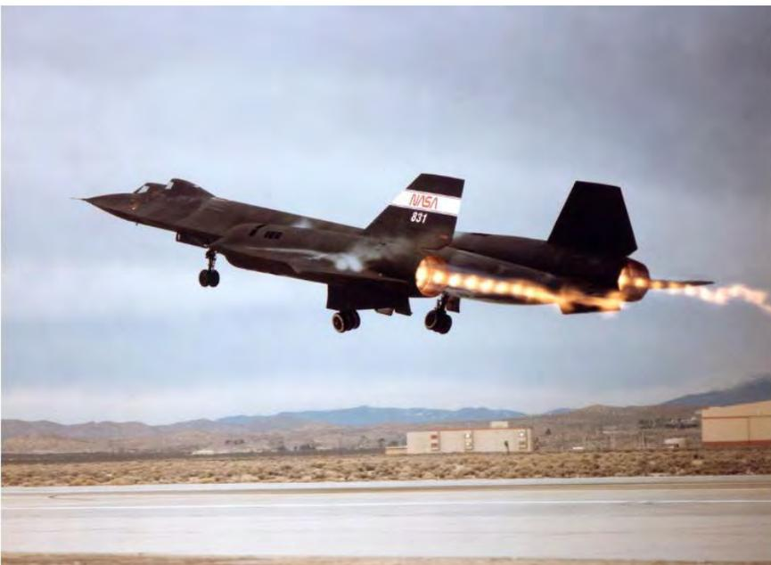
***The SR-71 was famous for the diamond pattern in its exhaust, which alternated between hot pockets of excess fuel that were ignited, and cooler sections of lower density. (DFRC/NASA)***
