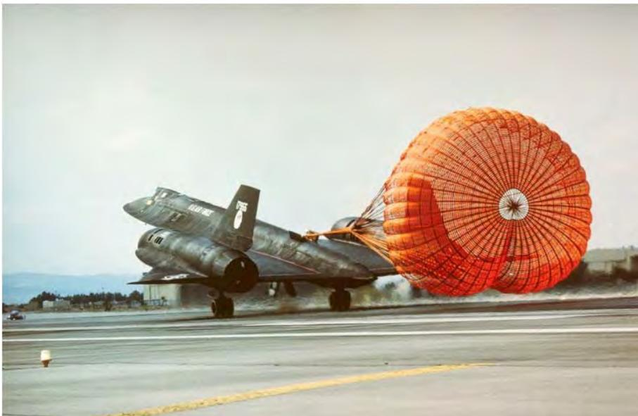
*Landing at about 170 mph, the SR-71 used a drag chute to relieve stress on the tires. After a chute failure, one Blackbird slammed off the runway and was destroyed. (Lockheed Martin)*
