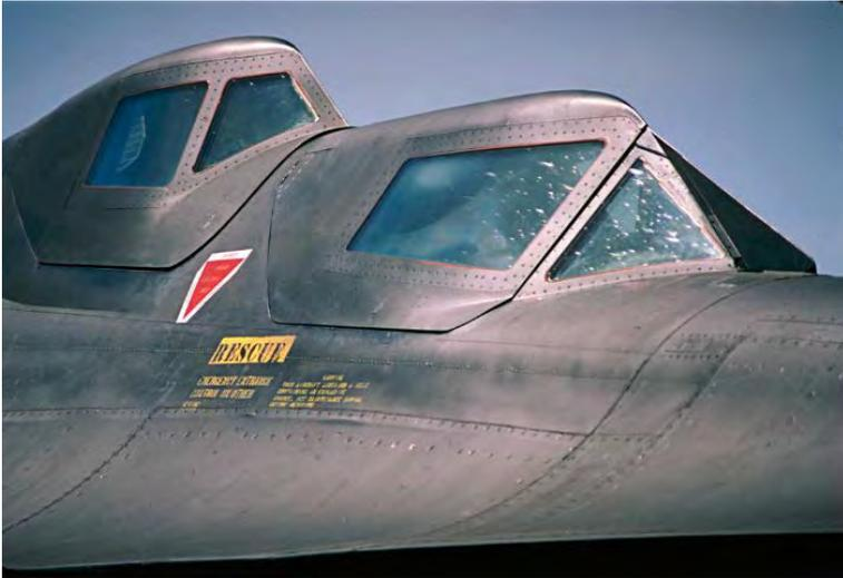
*High-frequency sound waves fused the quartz-glass outer windscreen directly to the titanium frame. At maximum Mach the windscreen exterior reached more than 600 degrees. Some pilots used the window as an ad hoc oven, pressing the squeeze tube that held their dinner against the glass to heat the food before eating. (Lockheed Martin)*
