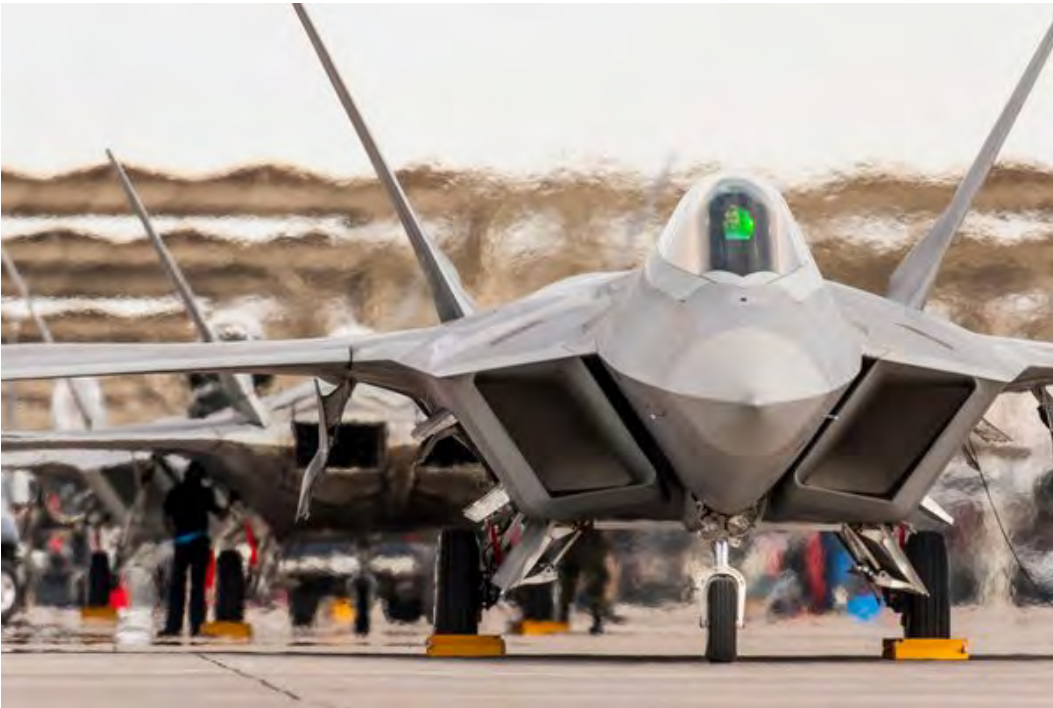
Chocked and lined up at Nellis, F-22s show off big intakes for dual engines, canted stabilizers, and a green glow on the canopy, light reflecting from a head-up display. (Richard VanderMeulen)
