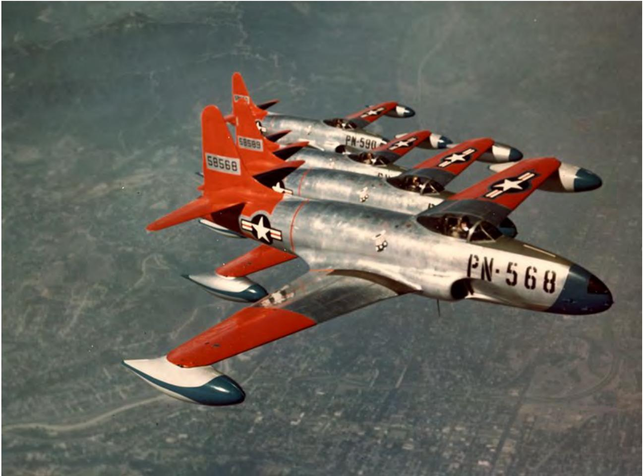
**The P-80 won the name Shooting Star for its speed: It was the first jet to exceed 500 mph in level flight. (NASM (SI-00064792))**
