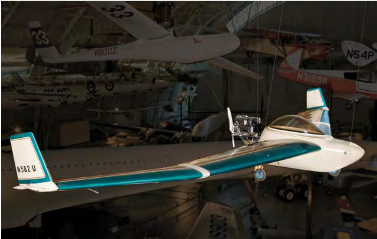
The Mitchell U-2 Superwing could be flown as a powered aircraft or a sailplane. Designer Don Mitchell estimated the kit could be built in 250 hours. (Dane Penland)
