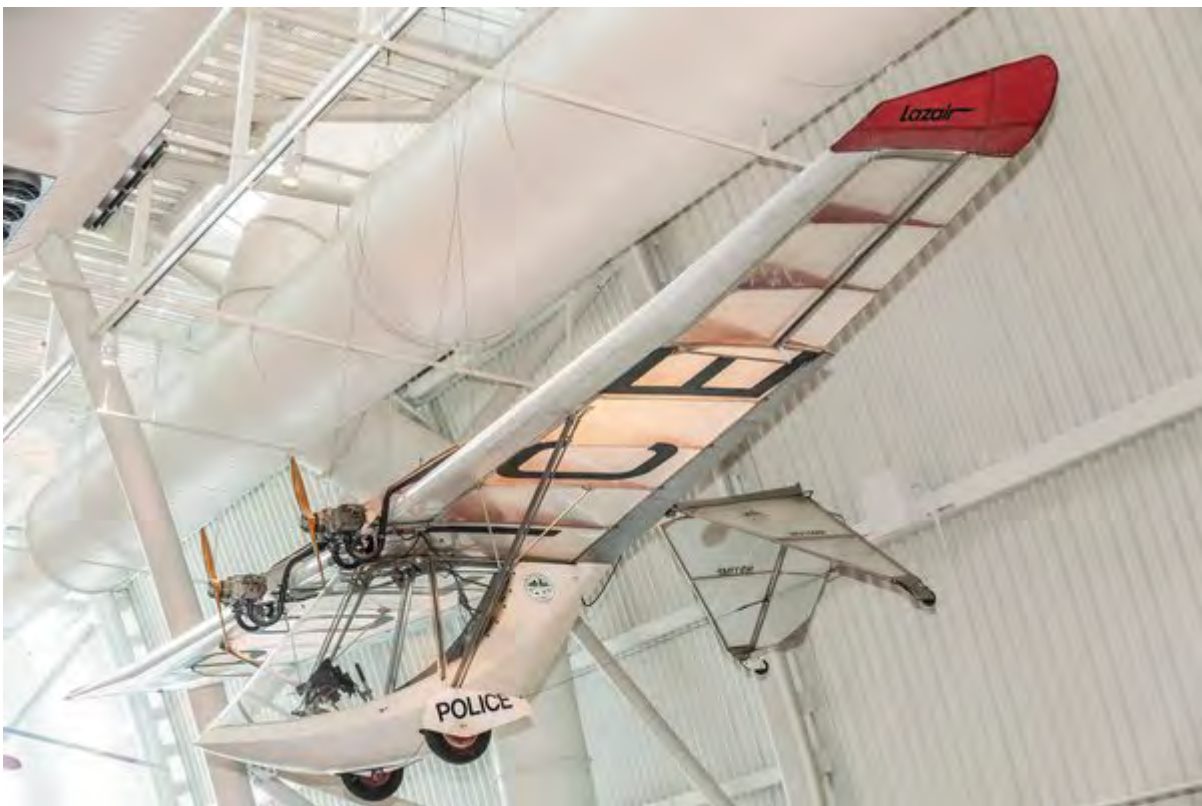
The Mitchell U-2 Superwing could be flown as a powered aircraft or a sailplane. Designer Don Mitchell estimated the kit could be built in 250 hours. (Dane Penland)
