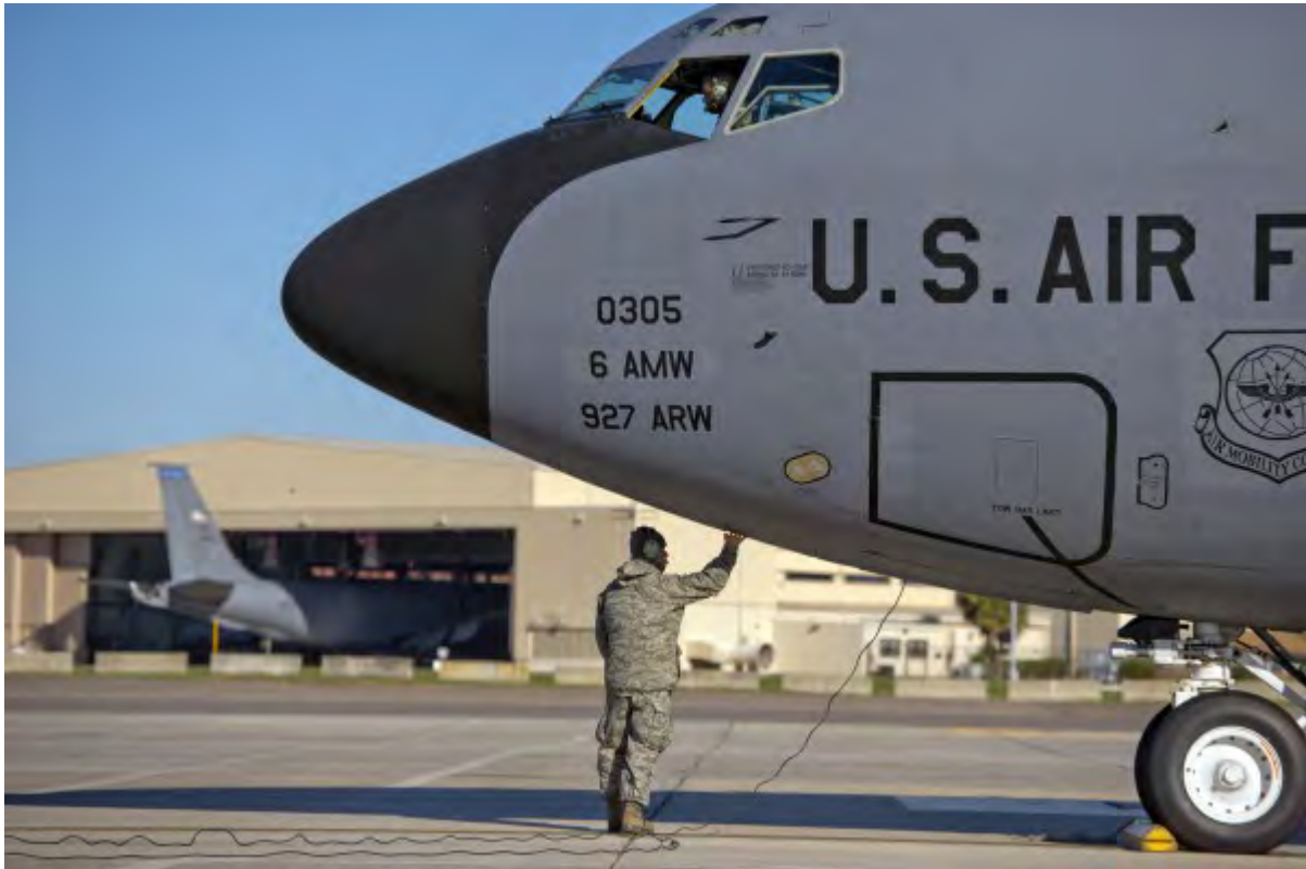
Tech. Sgt. Stephen Shin inspects KC-135 Stratotanker nose gear doors before taking off a training mission. Shin is a crew chief with the 927th Aircraft Maintenance Squadron at MacDill Air Force Base, Fla.
