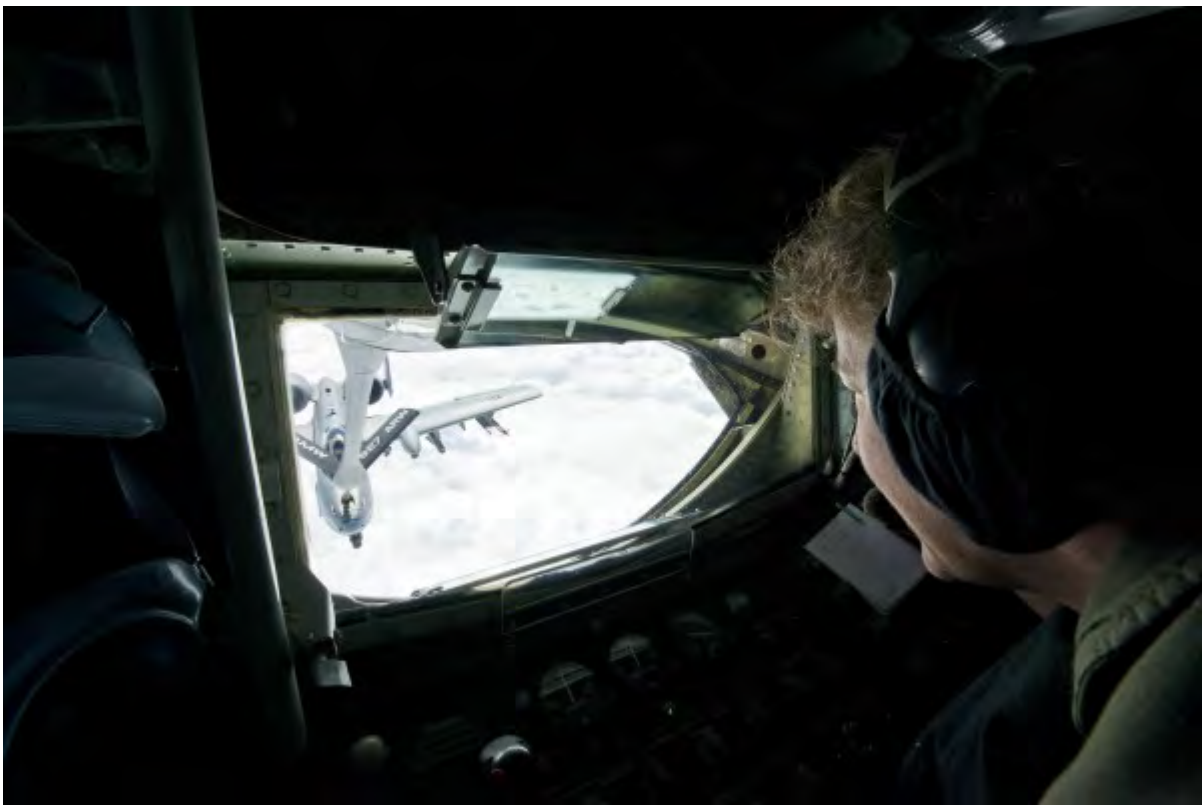
From a pod in the rear of a KC-135 Stratotanker, Master Sgt. Nancy Primm connects a refueling boom and transfers fuel to an A-10 thunderbolt II during a training mission over Valdosta, Ga. Primm is a boom operator with the 6th Mobility Wing at MacDill Air Force Base, Fla.
