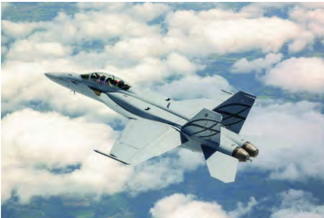
Boeing claims that its F/A-18 Advanced Super Hornet—fitted with new conformal fuel tanks (CFT) and an enclosed weapons pod (EWP)—will be able to outperform perceived threats well beyond 2030 in the anti-access, aerial denial environment. The advancement in capability is thanks to a suite of low-cost modifications, including enhanced stealth capabilities. Boeing Photo
