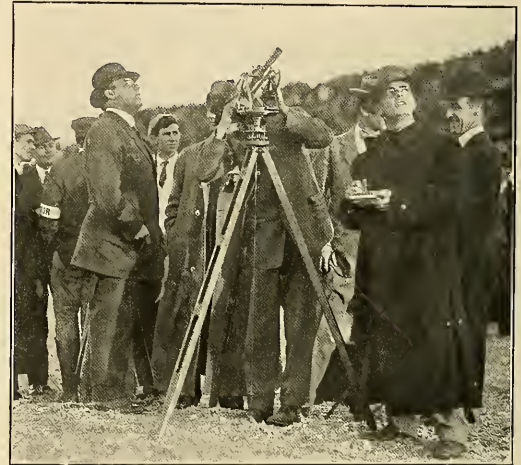
MEASURING ALTITUDE OF THE FLIERS WITH THE TRANSIT
