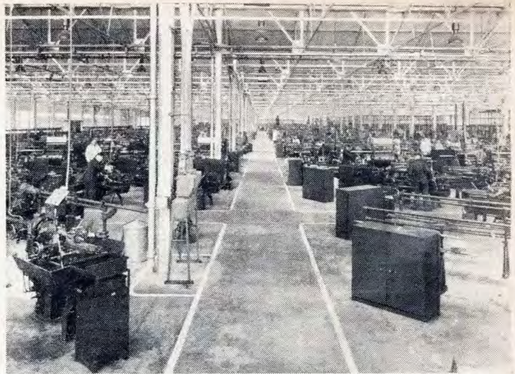
Lathes, shapers, drills and other workshop machines widely spaced in orderly rows on the floor of the new Rolls-Royce factory at Crewe, where Merlin aero engines are produced in rapid sequence for the R.A.F. and for export to France.
