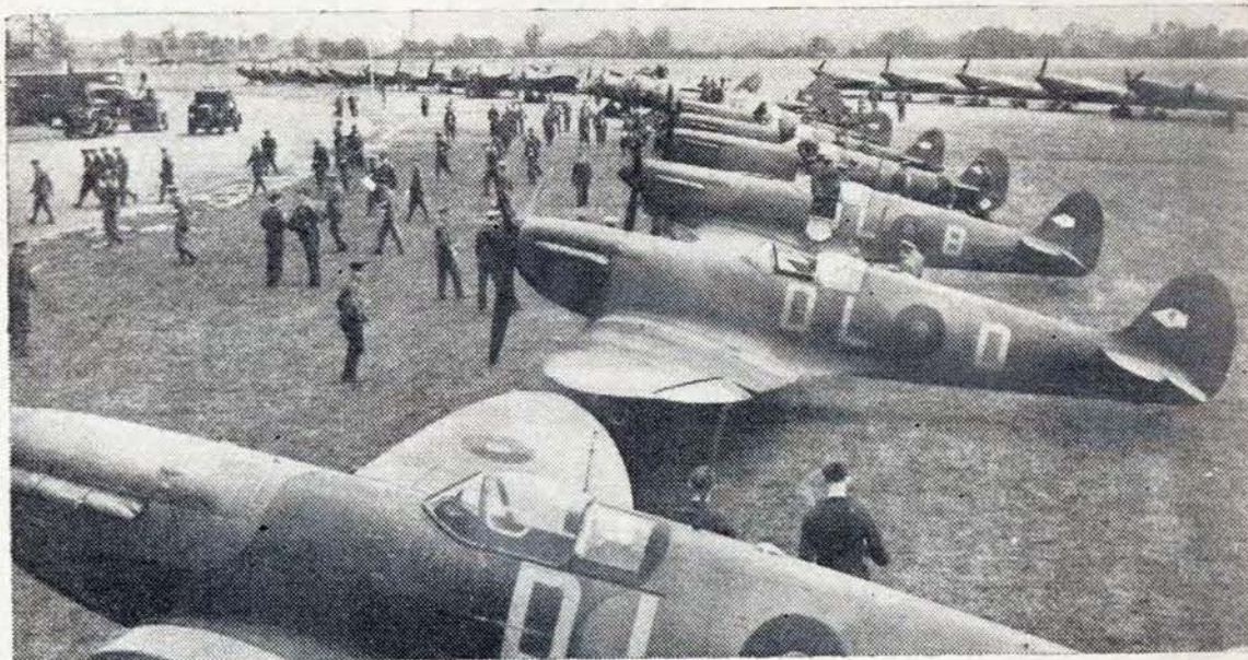
Supermarine Spitfires, with three-bladed variable-pitch airscrews, on parade at an R.A.F. station. Front cover shows a flight of Spitfires, credited with top speed of 367 m.p.h. and dived during tests at speeds in excess of 500 m.p.h.
