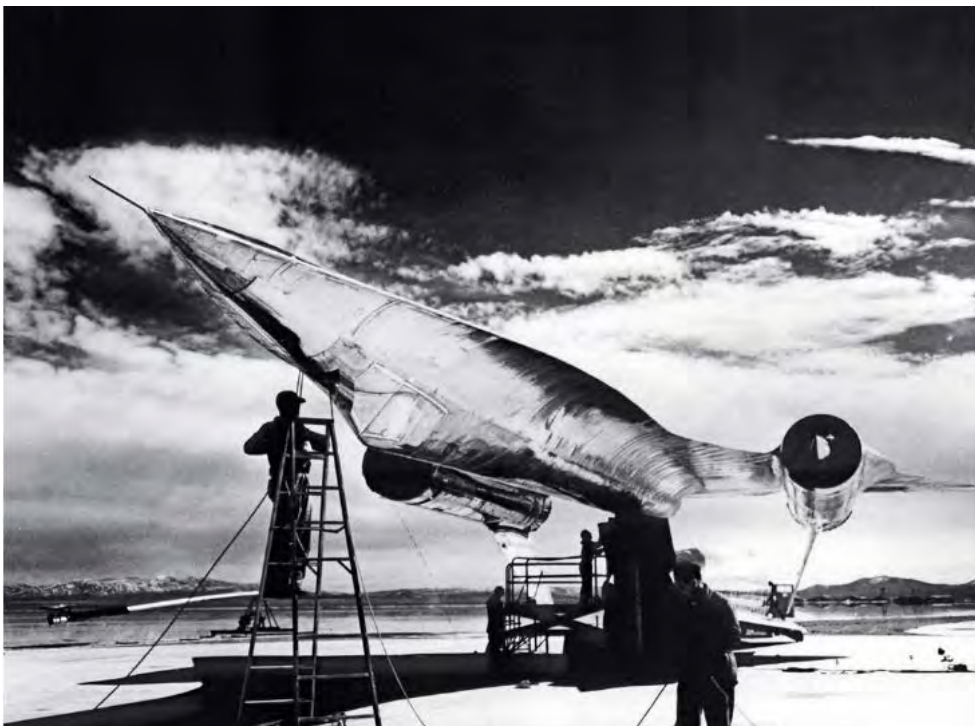
In the late 1950s, workers prepared an inverted A-12 prototype for tests to measure its radar cross-section. (Courtesy Roadrunners Internationale)
