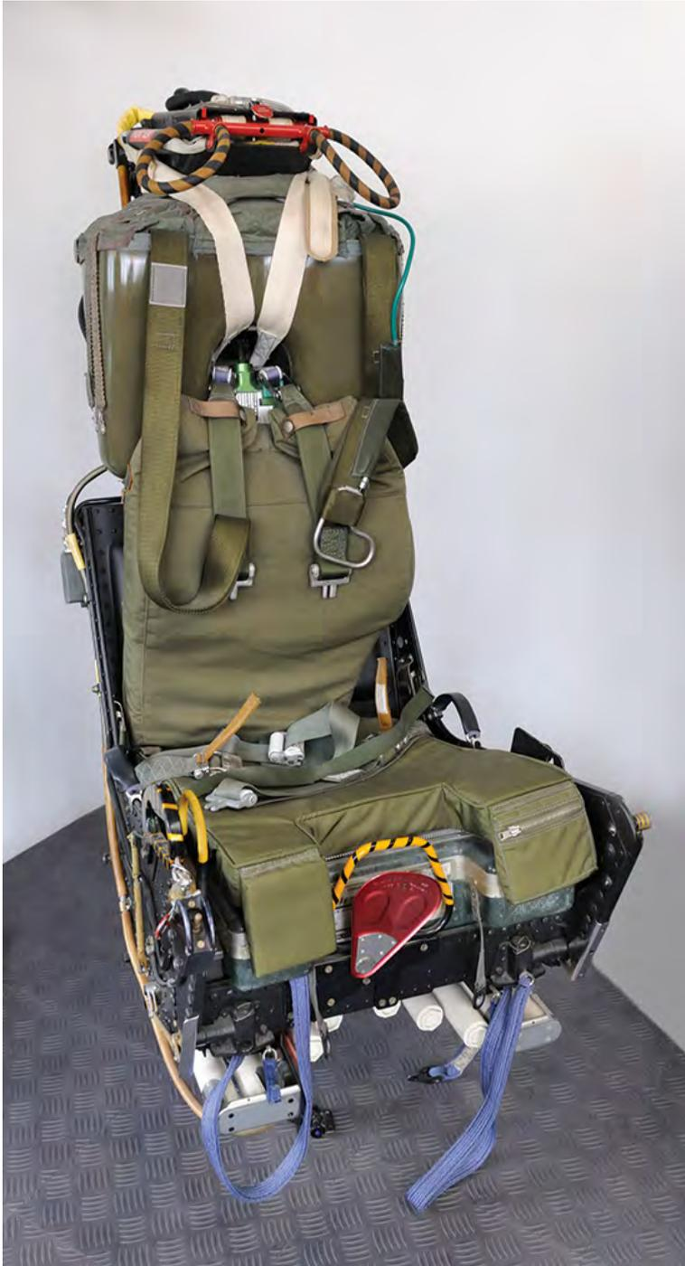
***The rocket-powered Mk. 7 ejection seat. Credit: Mark Wagner/Aviation-images.com***
