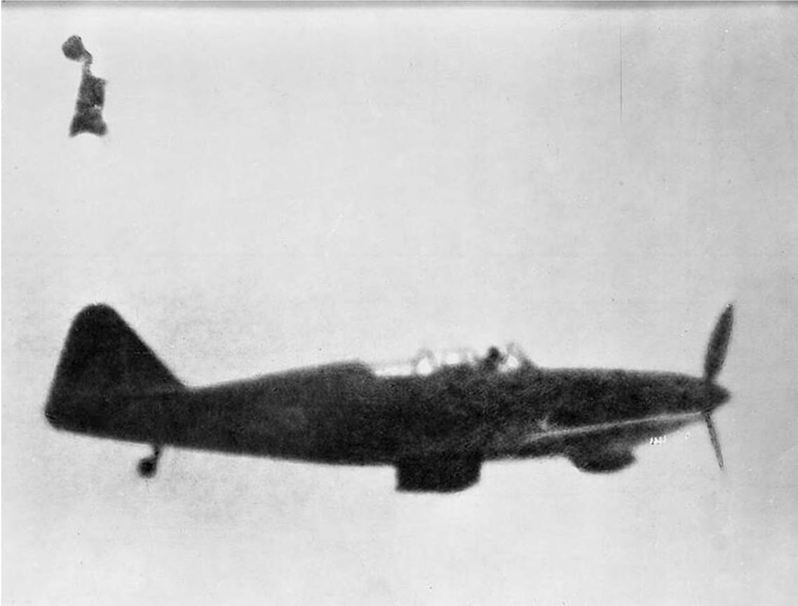
***The first dummy ejection of a Martin-Baker seat in flight was from a Boulton-Paul Defiant in 1945. Credit. Martin-Baker***
