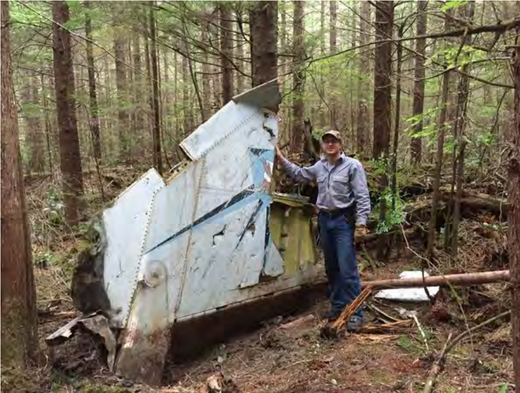
Austin Lunn-Rhue next to the F-106 vertical stabilizer with the partially intact tail flash of the 318th Fighter-Interceptor Squadron, the "Green Dragons." The forward aspect of the stabilizer is above his head; the rear aspect at his feet. (Courtesy Connor Heilman)
