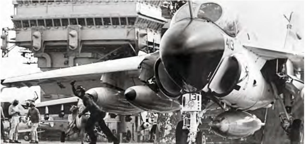
*On the USS Constellation late in 1968, a catapult crewman gives the signal that an A-6 is ready to launch. A centerline D-704 refueling store augmented the four drop tanks beneath the wings. The D-704's propeller, driven by wind in flight, powered a motor that extended and retracted its refueling hose. (Naval Historical Center)*
