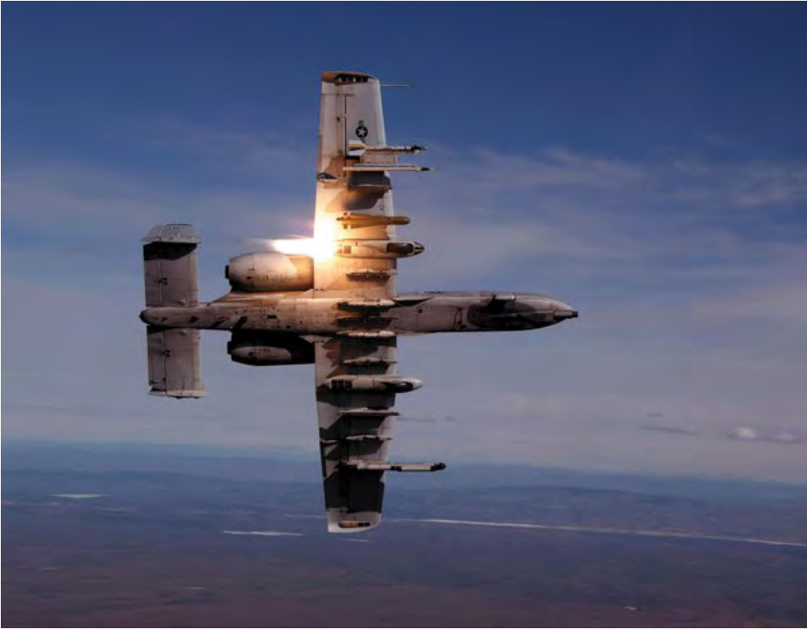
The Hog has 11 hard points on its underside for carrying an array of weapons. (USAF/Staff Sgt. Kenny Kennemer)
