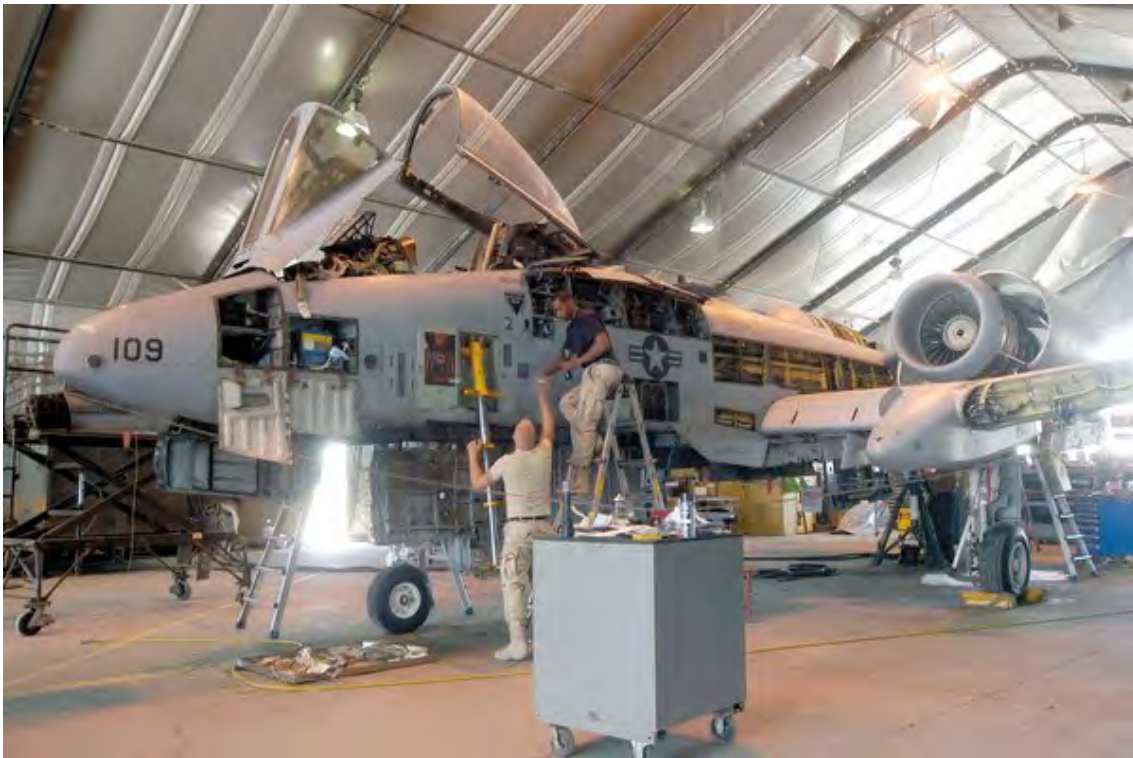
Shannon Hughes and Damon Johnson expose a Warthog's innards during an inspection at Bagram in 2006, when demand for close air support was high. (USAF/Maj. David Kurle)
