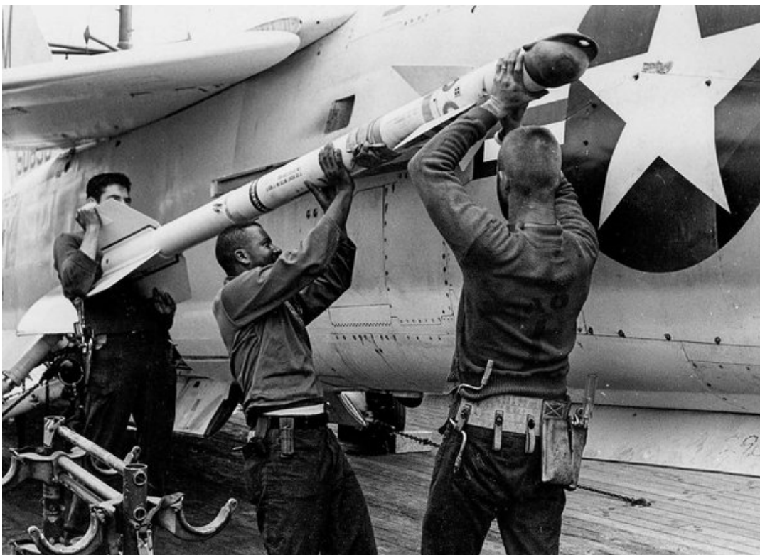
In the Tonkin Gulf in 1965, aviation ordnancemen of VF-194 load an AIM-9 Sidewinder onto an F-8 aboard the Ticonderoga. (National Naval Aviation Museum)
