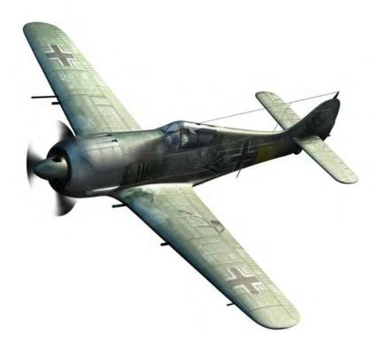
Firepower, agility, and the skill of its pilots made the Focke Wulf Fw 190 a feared opponent. Able to hit 400 mph downhill, the fighter carried four 20mm cannon in its wings and two 13mm machine guns in its cowl. (Paul Dimare)
