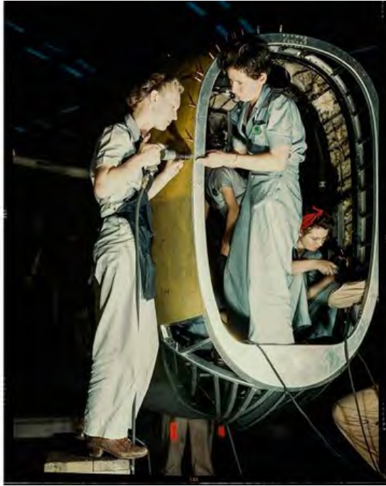
Riveter and bucker in the fuselage of a B-24 Liberator at a Consolidated Aircraft factory. Three other manufacturers built B-24s for the war: Douglas, North American, and Ford. (Library of Congress)
