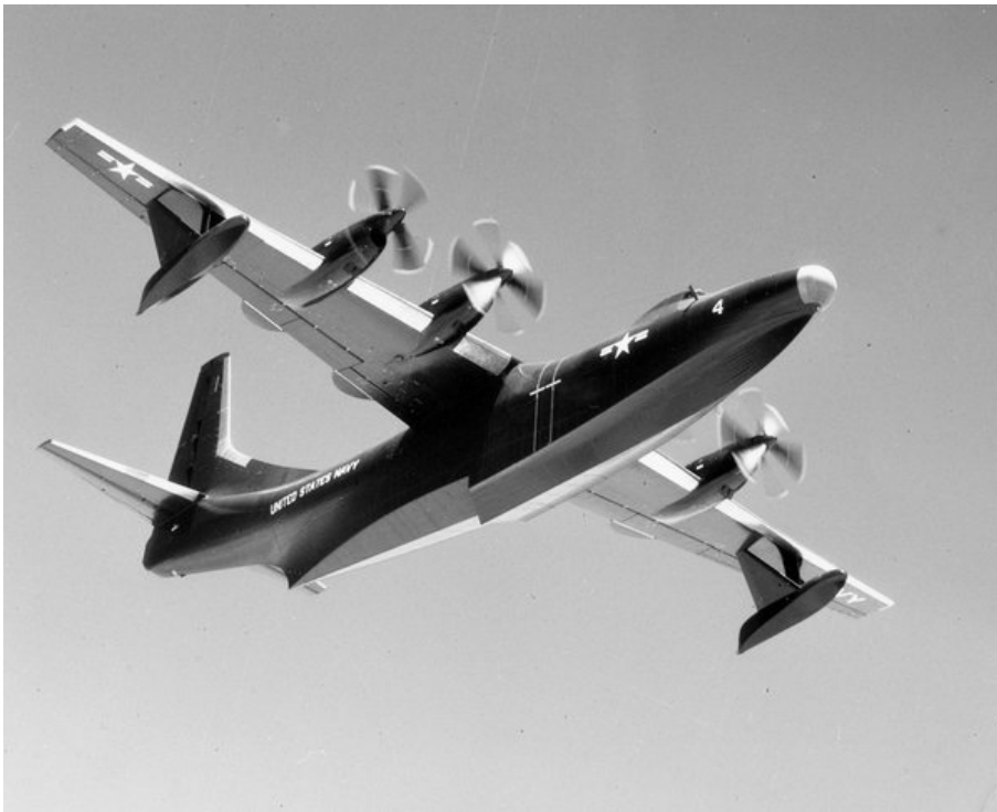
Problems with the contra-rotating propellers shortened the R3Y's service life for the Navy to barely two years. (San Diego Air & Space Museum)
