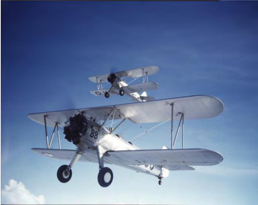
**★Boeing PT-17 Stearman. ★For military pilots during the 1930s and '40s, the primary trainer was the Stearman biplane, and the PT-17 was the most numerous of the more than 10,000 built by the Boeing Stearman company. It sported a serious radial engine making more than 200 horsepower to haul its nearly one-ton empty weight around the sky. (NASM)**
