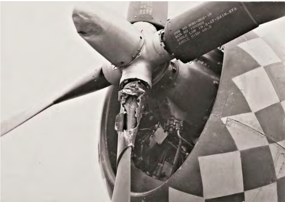
Strafing required concentration, lest pilots run into trees or powerlines, like the 353rd pilot flying this P-47. (AFHRA)
