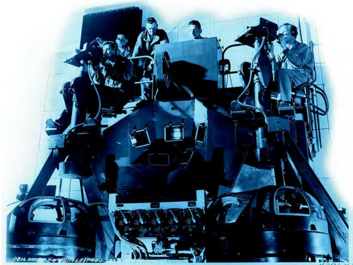
With stations for four gunners, the Waller trainer used multiple projectors (at center) to throw pictures of attacking airplanes onto a spherical screen. (Courtesy of Martin Hart/widescreenmuseum.com)
