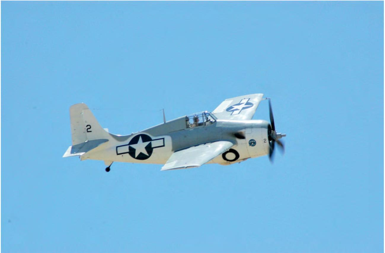
**An Eastern Aircraft FM-2 in flight; note the shorter cowl. Most surviving Wildcats are General Motors-built FM-2s, which are powered by the nine-cylinder Wright Cyclone engine. (Scott Schwartz)**
