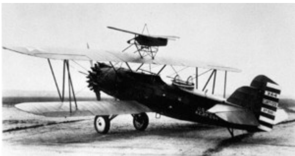
The US Army Air Service's GL-3 target drone ready for take off affixed to the top of the wing of a test aircraft at McCook Field. Photo Credit: USAF Museum
