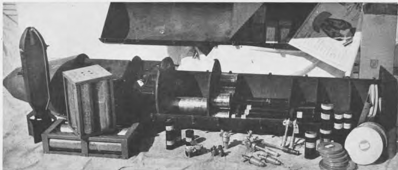
TORPEDO CONTAINER, PACKED WITH MANY TYPES OF BOMBS AND FUSES, EVEN A MOVIE PROJECTOR AND FILMS, IS CARRIED IN BOMB BAY OF TBF
