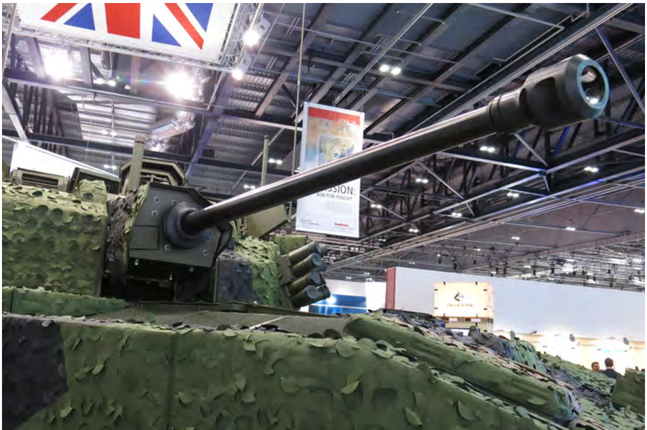
The new Ajax (Scout SV) armed with the 40mm Case Telescopic Cannon (CTC). Photo: Tamir Eshel, Defense-Update
