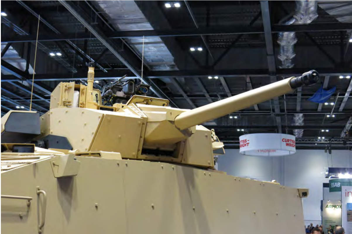
The 40mm turret being added to the VBCI-2 provides much higher lethality to the French AFV. The turret is manned by a crew of two, seated in the spacious capsule, surrounded by the vehicle's sensor displays that provide enhanced situational awareness in combat. The turret also mounts the 40mm CTC gun. Photo: Tamir Eshel, Defense-Update
