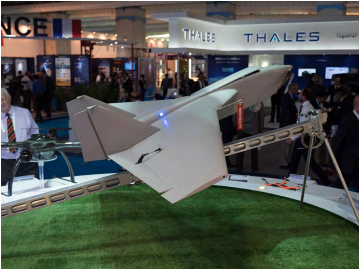
OIS also unveiled this twin tail Wavesight fixed wing UAV. It is launched from a catapult and retrieved using a parachute and airbags. Photo: Noam Eshel, Defense-Update
