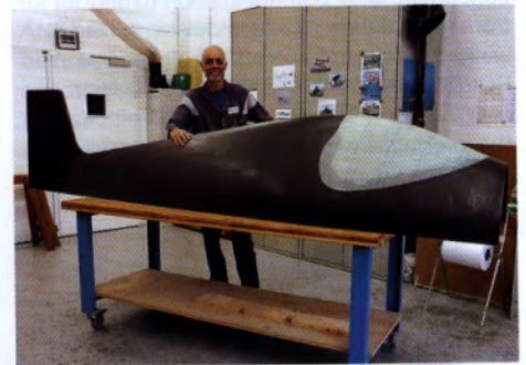
ABOVE: The all-new turtle deck before leaving the wind tunnel composite workshop
