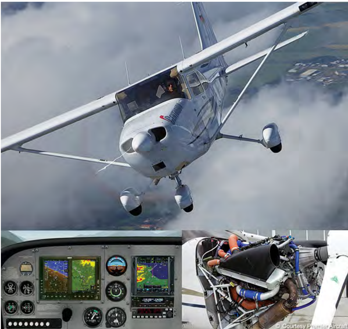
Premier Aircraft Sales Premier Edition 172 with Garmin panel and Centurion 2.0 liquid-cooled turbocharged diesel engine.
