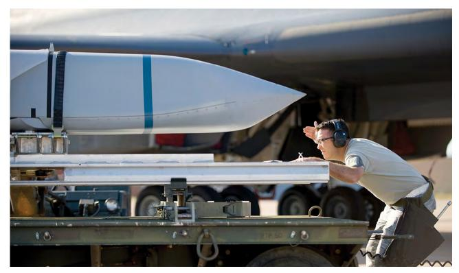
Lockheed's JASSM-ER can fly 500 nm and precisely strike land targets to within 3 m of the aimpoint, with an impact angle of 40 deg. nose low for soft targets and up to 70 deg. for penetration of hardened aircraft shelters or facilities. Credit: U.S. Air Force
