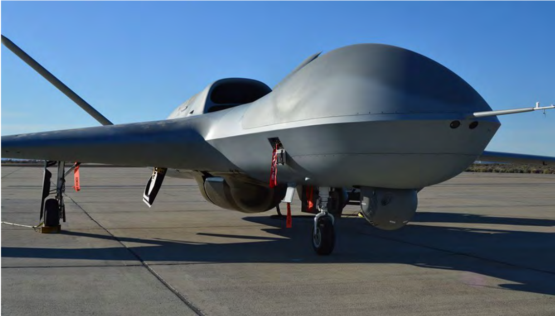
Sensors Unlimited's SYRES family MS-177 EO/IR multi-spectral reconnaissance payload was installed on General Atomics (GA-ASI) 'Predator C' Avenger stealthy drone for flight tests in January – February 2016. Photo: GA-ASI
