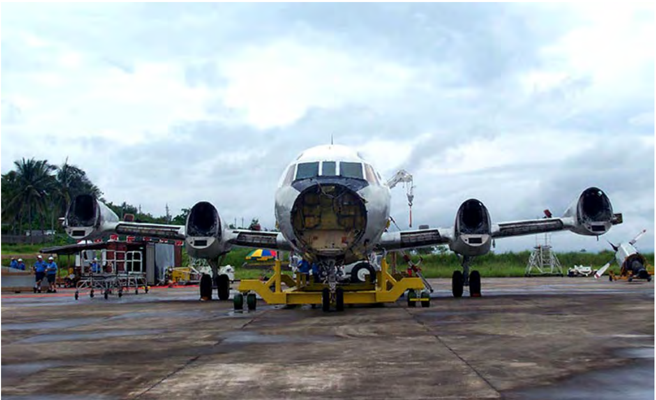
The Lockheed Martin Aeronautics Company's recovery team removed the four propeller-engine assemblies from the EP-3 at China's Lingshui air base, on Saturday June 23, 2001. Photo: Lockheed Martin Aeronautics Co., HO/AP Photo
