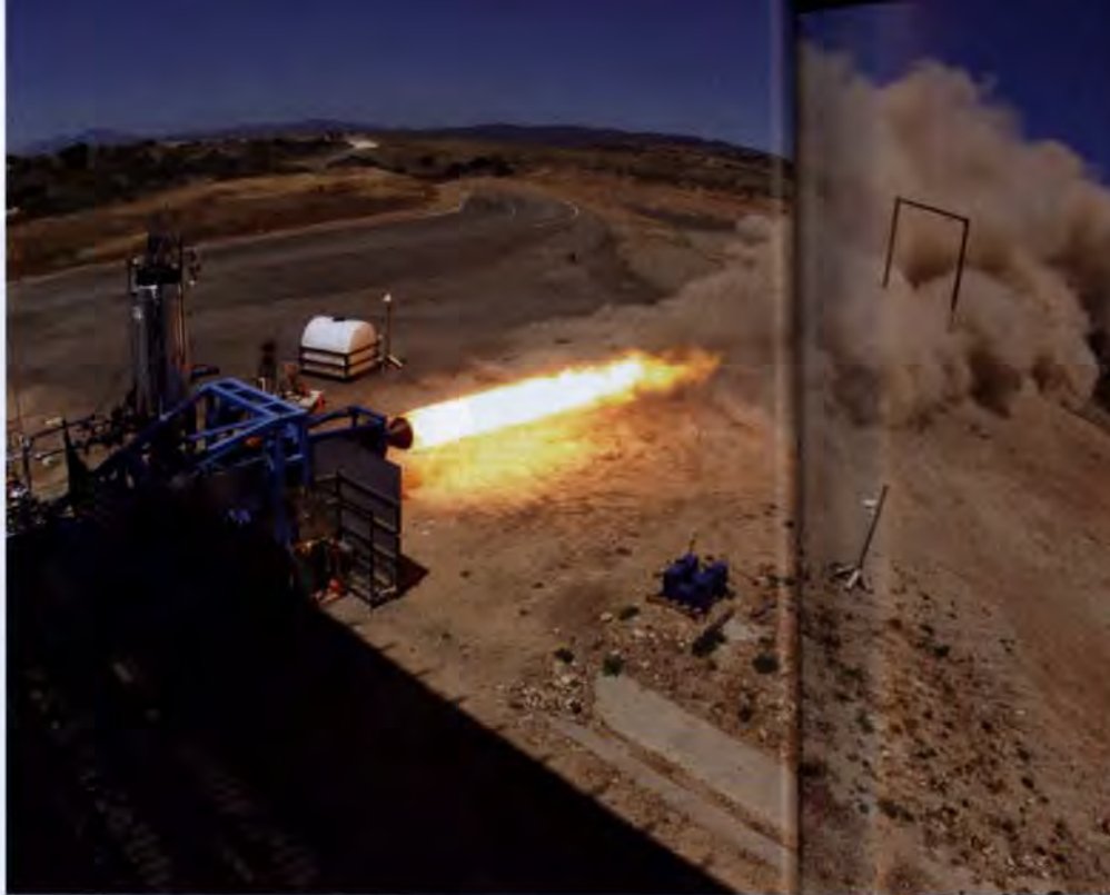
ABOVE: A view of a SpaceShipTwo hybrid rocket engine test firing by SpaceShipTwo builder Scaled Composites
