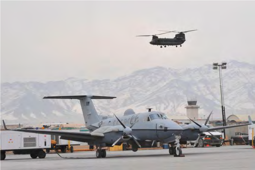
The MC-12 Liberty, a King Air stuffed with optical and other sensors that can detect the chemical signatures of explosives or heroin. (US Army)
