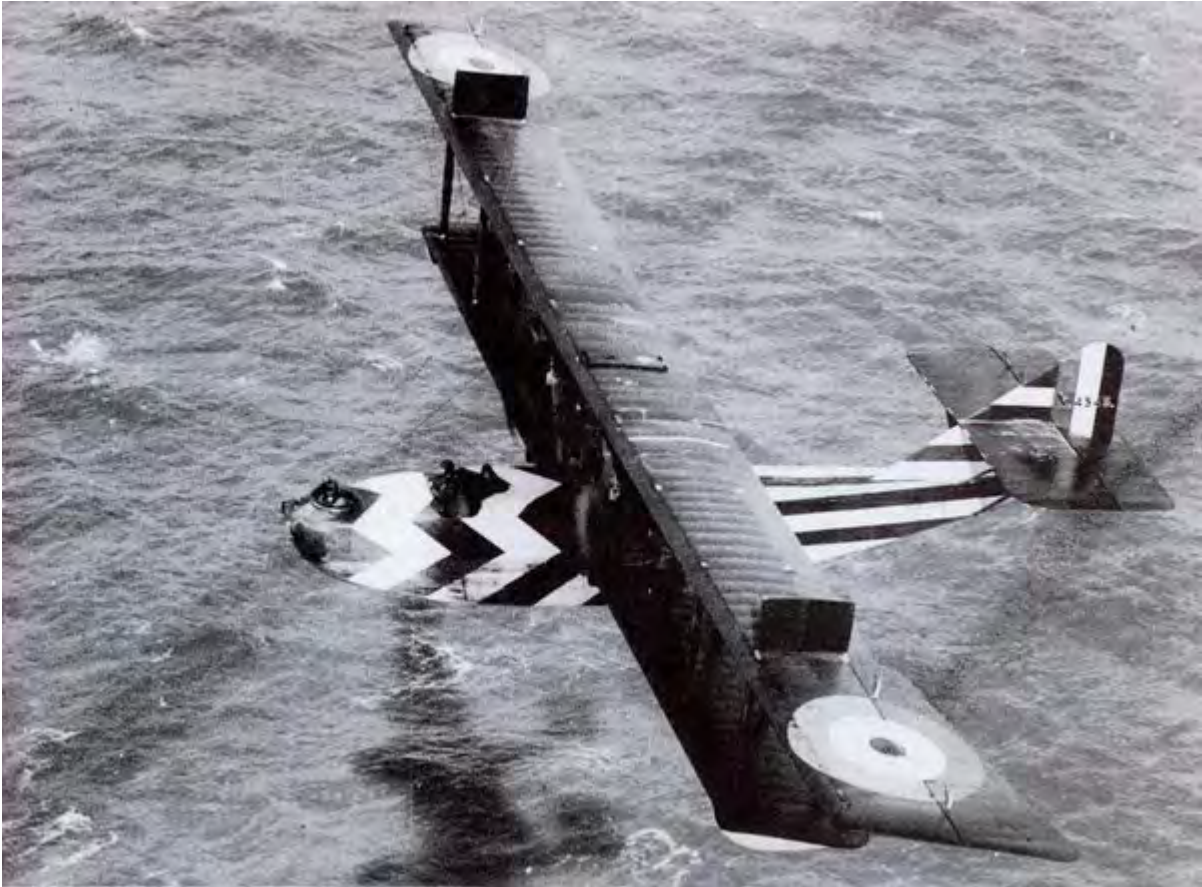
The bold patterns, such as the scheme on the Felixstowe, muddled the aircraft in the viewer's sight, making it difficult to shoot at. (Seawings)
