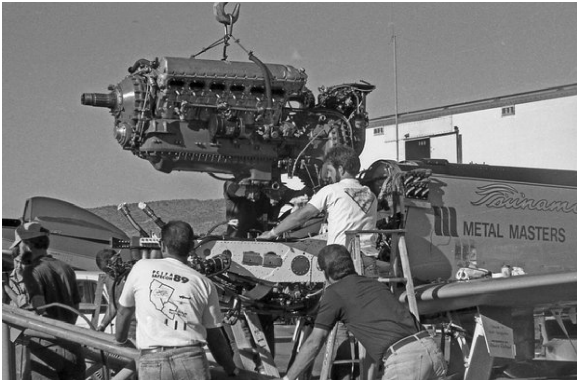
Tsunami was built around a Rolls-Royce Merlin engine. Seventy years ago Merlins were state of the art, and they're still the gold standard of race engines. Most Reno Unlimited racers use one. (Tim Weinschenker)
