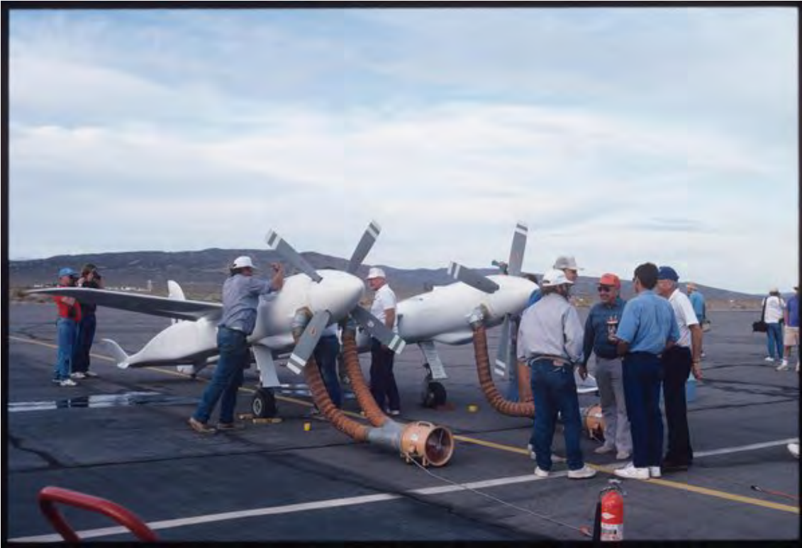
Pond Racer's methanol-fueled engines needed meticulous care: Among other headaches, the crew had to race to attach cool-air blowers to each engine immediately upon shutdown. (Don "Bucky" Dawson)
