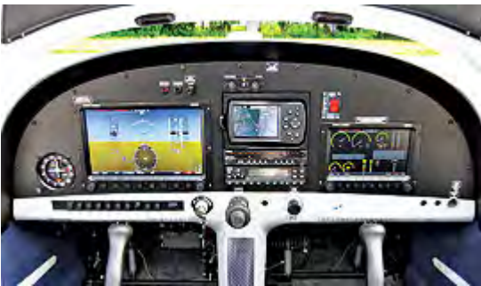
Dynamon SkyView Innovative avionics, such as Dynamon's SkyView panel, are commonplace in LSA since certification isn't required.
