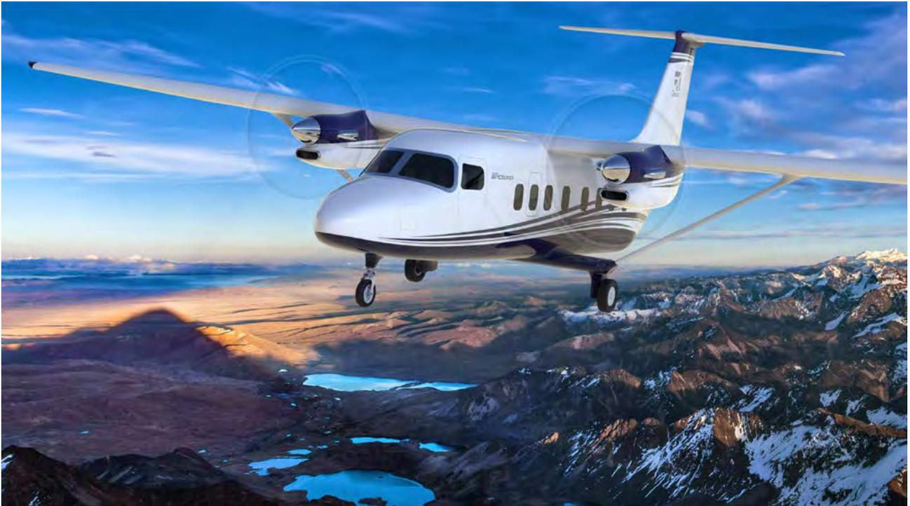
***Pratt & Whitney PT6 turboprop engines will power the SkyCourier.***
