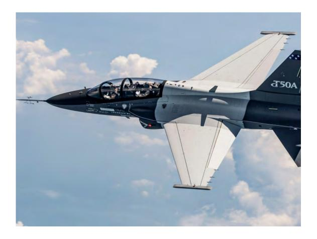
T-50A is an advanced trainer jet aircraft developed jointly by Lockheed Martin and Korea Aerospace Industries (KAI) for the US Air Force's T-X Advanced Pilot Training (APT) competition. It is an advanced version of the T-50 trainer aircraft.
