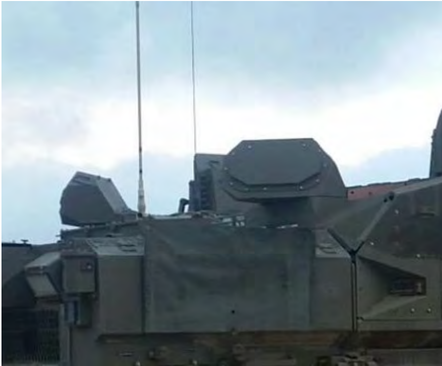
These two Windguard AESA radars are part of the 360 degrees sensor of the Trophy system. They provide the situational picture, threat detection and fire control cueing for the Trophy APS system. Photo: IMOD
