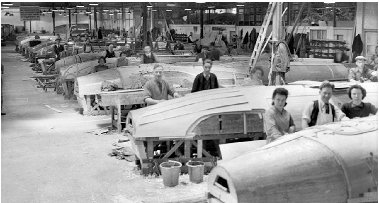
One of the places where the RAF's wooden Mosquito fighter bomber is made is at the Walter Lawrence & Sons joinery works in Sawbridge, Hertfordshire.
