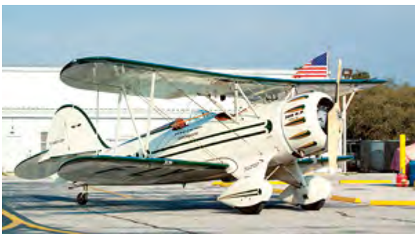
The radial Jacobs R-755 is upgraded to provide 300 hp on takeoff.
