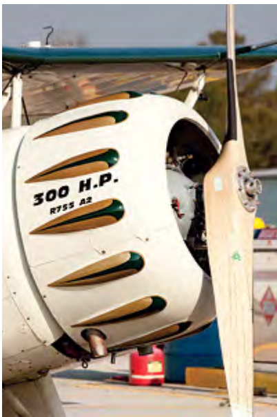
The radial Jacobs R-755 is upgraded to provide 300 hp on takeoff.
